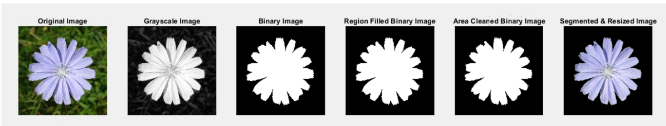
Figure 2.2 Segmentation Process for Chicory using Blue Color Channel
